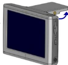
GPS Antenna Up (Parallel to the Ground)
