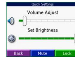
Touch **Lock** to prevent accidental screen taps. To unlock the screen, press the **Power** button and touch **Unlock**.
