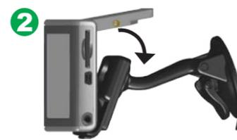
Open the antenna. Fit the bottom of your nüvi into the cradle. Tilt your nüvi back until it snaps in place. If necessary, rotate the cradle.
