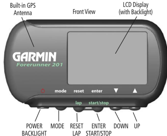
The Forerunner has been designed to comfortably fit your wrist. For best performance, wear the Forerunner like a watch, with the top face of the unit oriented towards the sky. A strap extension provides additional length and easily attaches to the existing strap.
