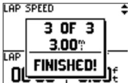
Once Interval Training has started, the Forerunner automatically changes to the Timer Mode, showing your Lap Speed, Lap Time, and Lap Distance. An audible alarm sounds when you have reached your rest time or distance period. A Rest Banner displays showing the time or distance of your rest period. During the rest period, another audible alarm sounds when you are within 5 seconds or 20 meters of resuming your workout.
